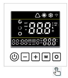
Hold the button for 3 seconds to enter the setting of Timer ON & Timer Off groups.
